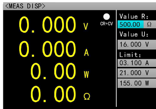
Chart 2.6.5 Constant Resistance-Constant Voltage Measurement Mode
